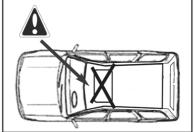
Do not open the sunroof when these roof bars are fitted
