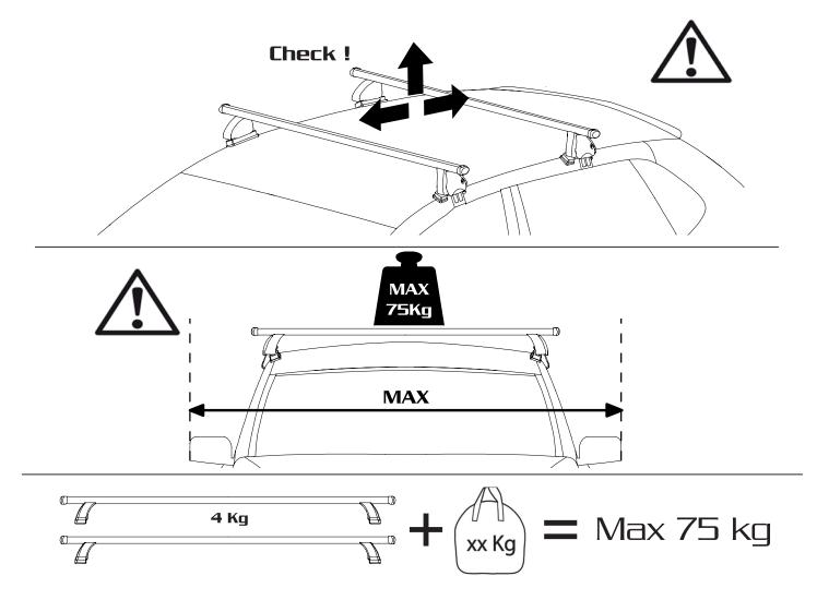
$\operatorname{\textbf{EN}}$  : Not exceed the total weight permitted on the vehicle roof
