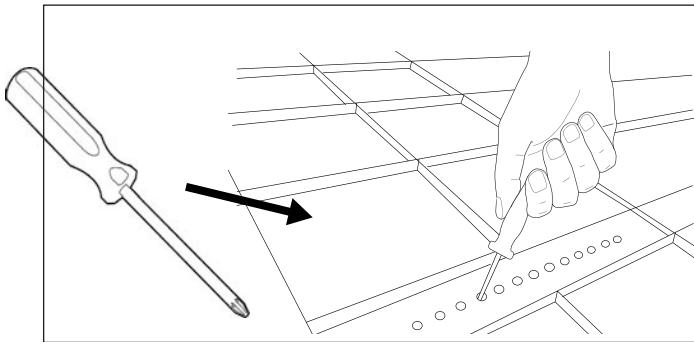
Remove the box from the bars and place on the ground. Now using one of the U-Bolts as a template, mark the hole/ indent nearest to the front mark made earlier (but not beyond) at the front of the bar. Also mark the hole/ indent which lines up with the rear of the U-Bolt. Using either a screwdriver or a drill make holes previously marked when using the U-Bolt. Do not drill or try to make the holes whilst box is on the vehicle, this may cause damage to the vehicle.
