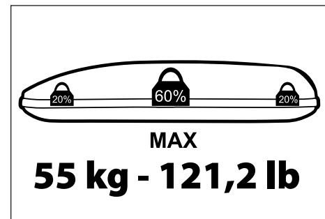
When loading the roof box ensure that the weight is evenly distributed as per above diagram. The contents should be fixed or strapped down to stop any movement. The box lid must always be closed and secured correctly using the front safety lock and key.
