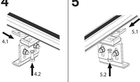
Place the bar onto the mounting brackets, insert the bar locator plate. Insert the 13mm headed bolt & washer from below, to hold in place.
