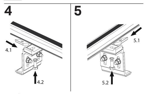
Place the bar onto the mounting brackets, insert the bar locator plate. Insert the 13mm headed bolt & washer from below, to hold in place.
