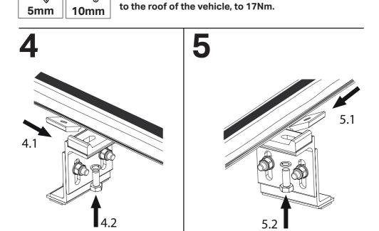
Place the bar onto the mounting brackets, insert the bar locator plate. Insert the 13mm headed bolt & washer from below, to hold in place.
