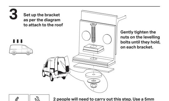
Allen key and 10mm spanner to install the 6 brackets
