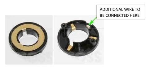
YOU WILL NEED TO MAKE UP A NEW WIRING CONNECTION TO MAKE THE HORN WORK WHEN FITTING THE MOUNTNEY BOSS.
