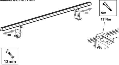
Using a spirit level, adjust mounting brackets until level left to right & front to rear. Once level fully tighten the levelling bolts/nuts, using the 13mm spanner to 17Nm.
