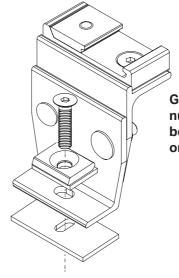
Gently tighten the nuts on the levelling bolts until they hold, on each bracket.
