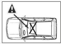
Do not open the sunroof when these roof bars are fitted
