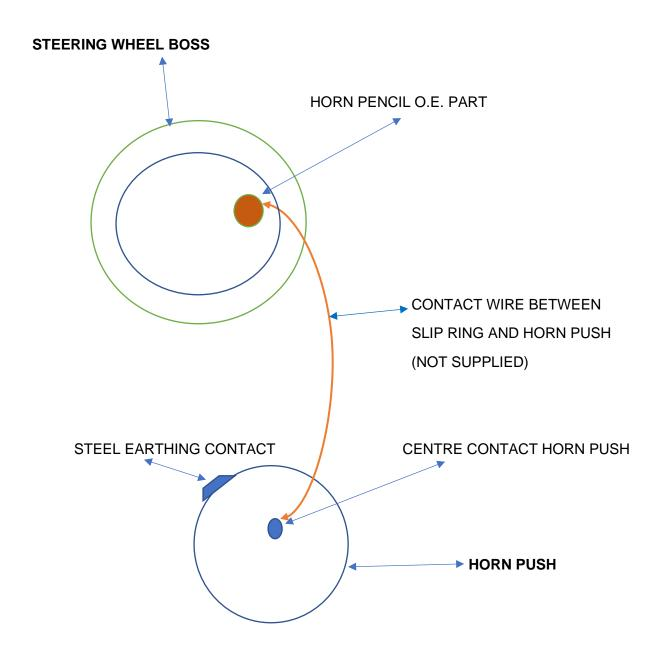
YOU WILL NEED TO MAKE UP A WIRE BETWEEN THE TOP OF THE HORN PENCIL AND THE HORN PUSH CENTRAL BRASS CONTACT.
