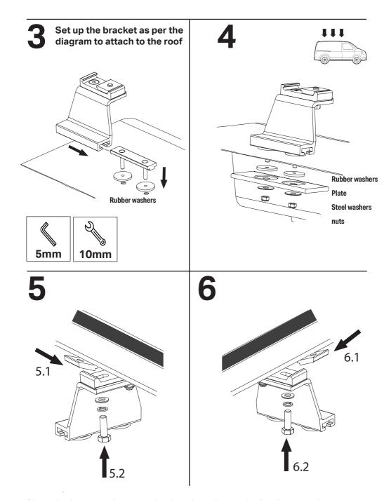
Place the bar onto the mounting brackets, insert the bar locator plate. Insert the 13mm headed bolt & washer from below, to hold in place.
