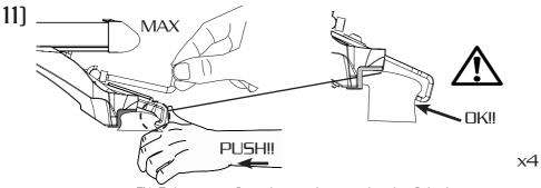
EN: Tighten your feet alternately on each side of the bar
