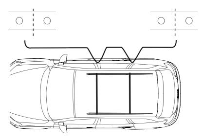
If the vehicle is equipped with original fix points, place the bars in the middle of them.
