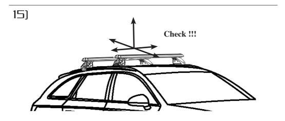
Before driving and at regular intervals during your journey, check that all securing screws and foot attachments are fully tightened. Additionally ensure that the load is fastened securely.
