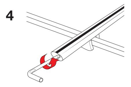
Using the Allen key, tighten the foot clamps alternately onto each side of the roof bar.
