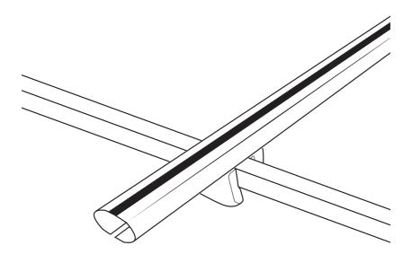
Place the roof bars onto the vehicles original rails, ensuring the positional guidance in step 2 is followed.
