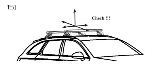
EN: Before starting, ALWAYS check that bars and cargo are correctly tightened, if necessa¬ry, repeat assembly or check it with an authorized dealer.
