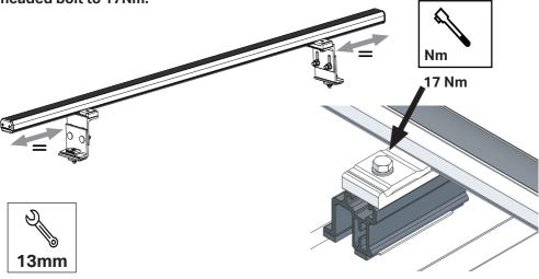
Once fully tightened, fit the supplied covers to the nut & bolt heads.
