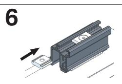
Place the bar onto the mounting brackets, insert the bar locator plate. Insert the 13mm headed bolt & washer from below, to hold in place.
